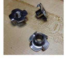
the inside of the countersink hole. Remove the receiver, and slightly pre-drill those indentations. This gives the claw a place to sink in without forcing apart the wood and thus avoids the end caps from splitting when you seat the receivers.
