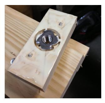
Now apply glue to the end cap, place back on the end of the board, such that the screws drop into their pre-hammered divits, and tighten the screws till the cone screw heads countersink into the end of the endcap, pulling it against the board, squeezing out glue and making a tight fit.
