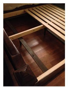
in length for my king frame. The boards started out as 1x4 x 8feet at the big-box home center. Remember you need to leave room for bolting the end boards on when deciding how long to cut these weight bearing boards.
